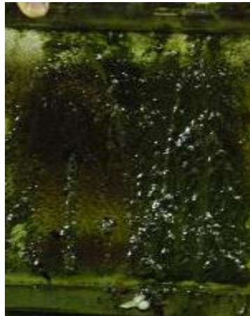
Figure 5. Membrane populated with microalgae.
