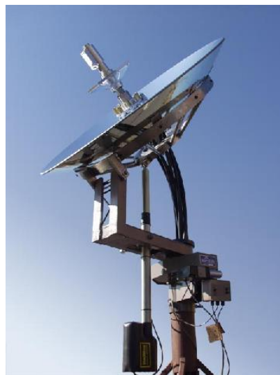
Figure 3. Solar Collector mounted above pilot-scale bioreactor.
