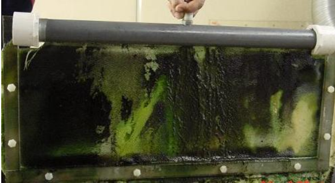
Figure 2. Populated substrates showing capillary transport of water.
