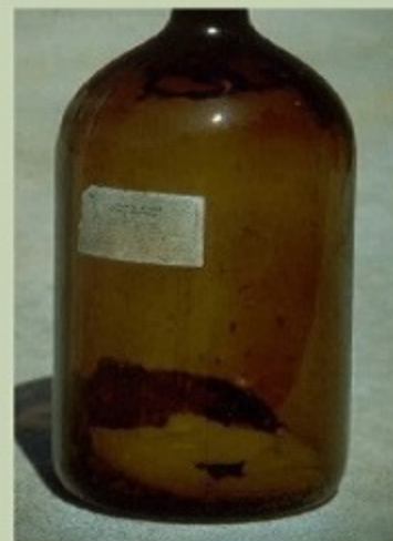
One gallon bottle with crystals from Isopropyl Ether
