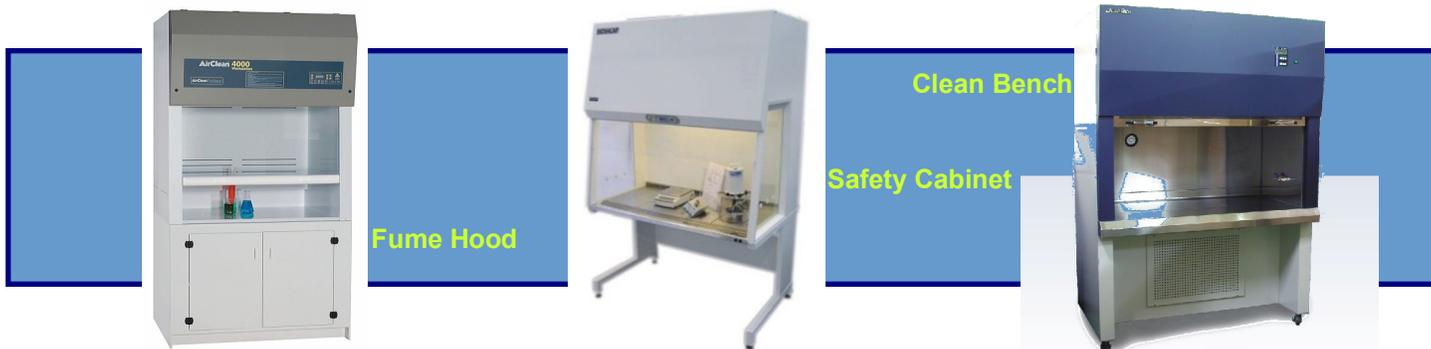
Fume hoods, biological safety cabinets and clean benches are three common laboratory ventilation devices designed to protect the worker and/or the experiment. It is important to know when each is necessary and under which conditions each should be used.
