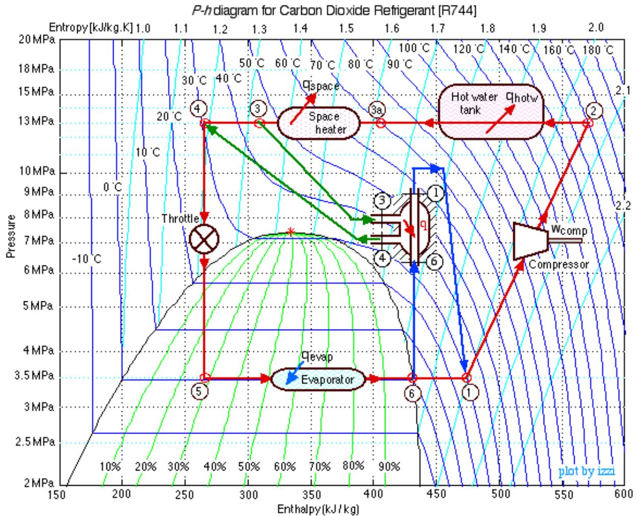
Figure 8 – Pressure-enthalpy ( $P-h$ ) diagram of carbon dioxide
