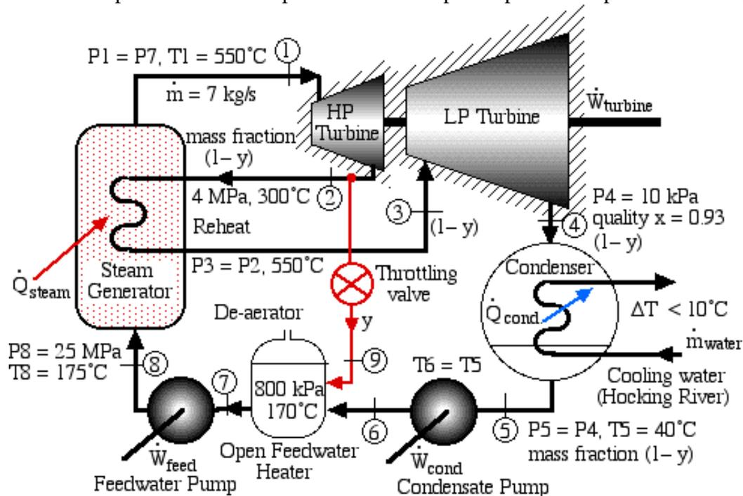
Figure 1 - Super-critical Steam Power Plant Example
