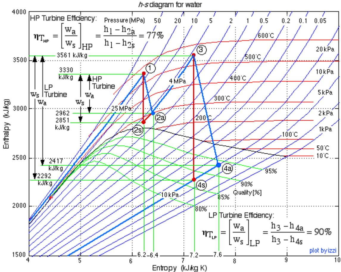
Figure 3 – Enthalpy-entropy (*h-s*) Mollier diagram for water-steam
