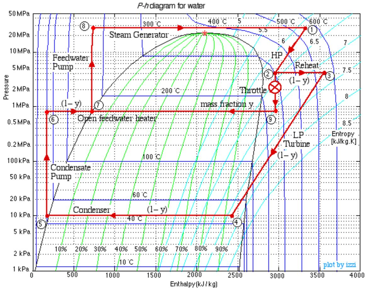
Figure 2 – Pressure-enthalpy ( $P-h$ ) diagram for water-steam
