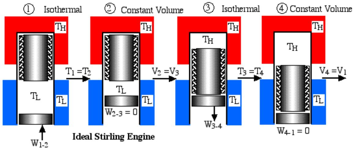
Figure 5 - Ideal Stirling cycle heat engine
