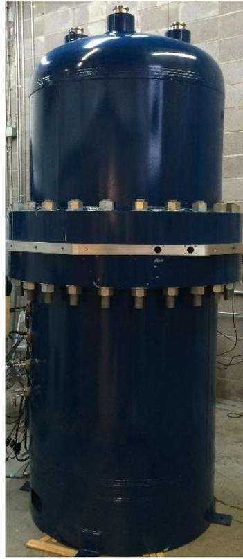
*Fig 5) left: 25kW ThermoHeart® Engine. The penetrations in the upper pressure vessel are the thermal heat transfer oil inlets and outlets. The heat rejection fluid is circulated through the center aluminum plate.*
