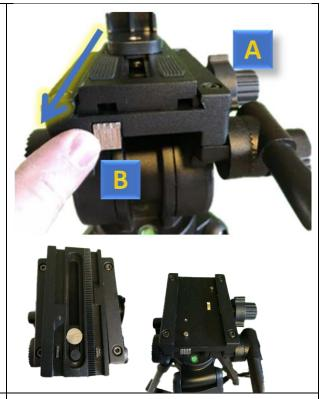
Insert the screw and peg on the mounting plate into the matching sockets on the bottom of the camera (a flat screwdriver or coin may make this easier).
