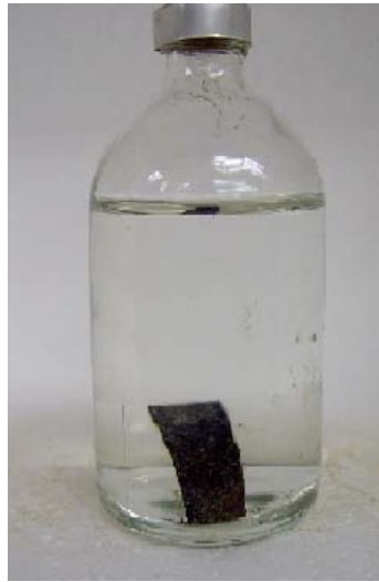
FIGURE – 1. X65 coupon in an anaerobic serum bottle
