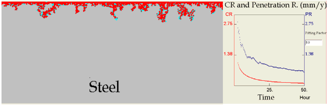
Figure 12. Surface morphology and the trend of the corresponding uniform corrosion rate (lower curve denoted CR) and localized penetration rate (upper curve denoted PR) as predicted by 2-D model at 28 ppm Fe 2+ , 0.54 bar pCO 2 , 80 °C, pH 6.6, and 1 m/s.
