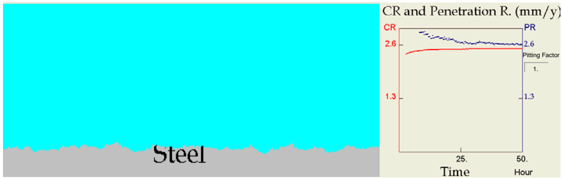
Figure 8. Surface morphology and the trend of the corresponding uniform corrosion rate (lower curve denoted CR) and localized penetration rate (upper curve denoted PR) as predicted by 2-D model at 0 ppm Fe^{2+} , 0.54bar pCO_2 , 80 °C, pH 6.6, and 1m/s.
