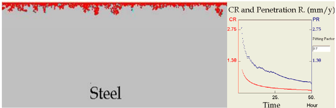
Figure 13. Surface morphology and the trend of the corresponding uniform corrosion rate (lower curve denoted CR) and localized penetration rate (upper curve denoted PR) as predicted by 2-D model at 30 ppm Fe 2+ , 0.54 bar pCO 2 , 80 °C, pH 6.6, and 1 m/s.
