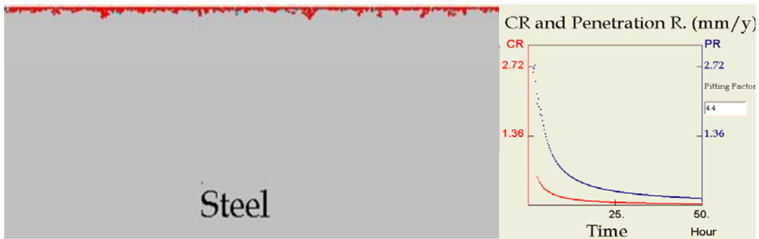
Figure 14. Surface morphology and the trend of the corresponding uniform corrosion rate (lower curve denoted CR) and localized penetration rate (upper curve denoted PR) as predicted by 2-D model at 50 ppm Fe 2+ , 0.54 bar pCO 2 , 80 °C, pH 6.6, and 1 m/s.
