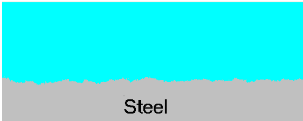
Figure 1. Two samples of simulated metal surface morphology following rapid uniform corrosion without any film precipitation. Original Pots (14) algorithm was used.
