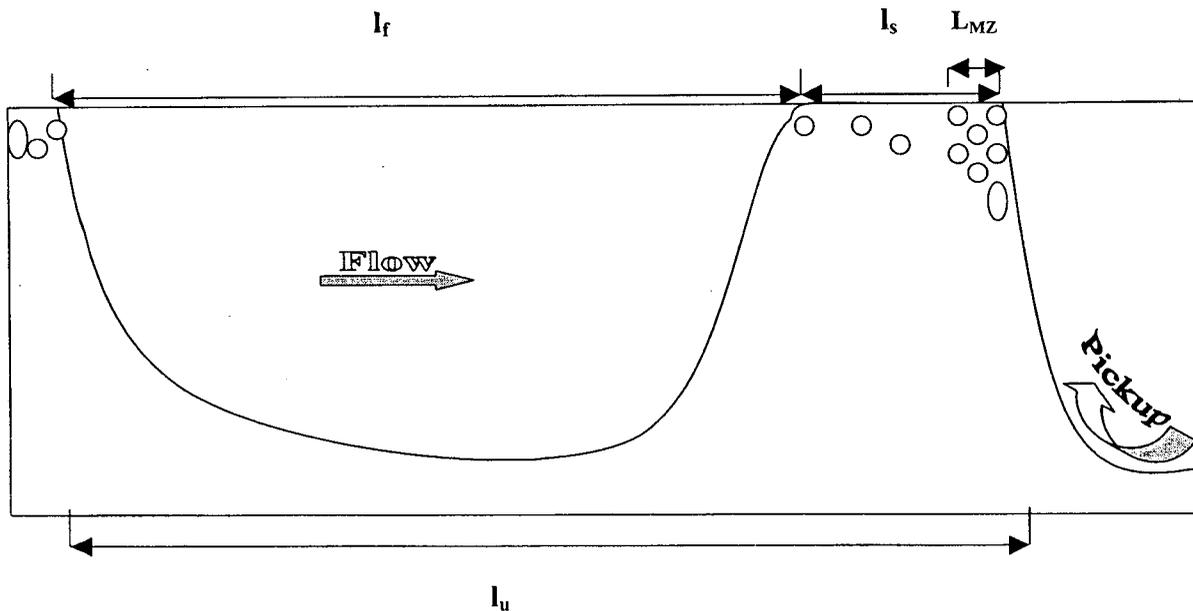
Figure 2 Schematic diagram of a stable moving slug
