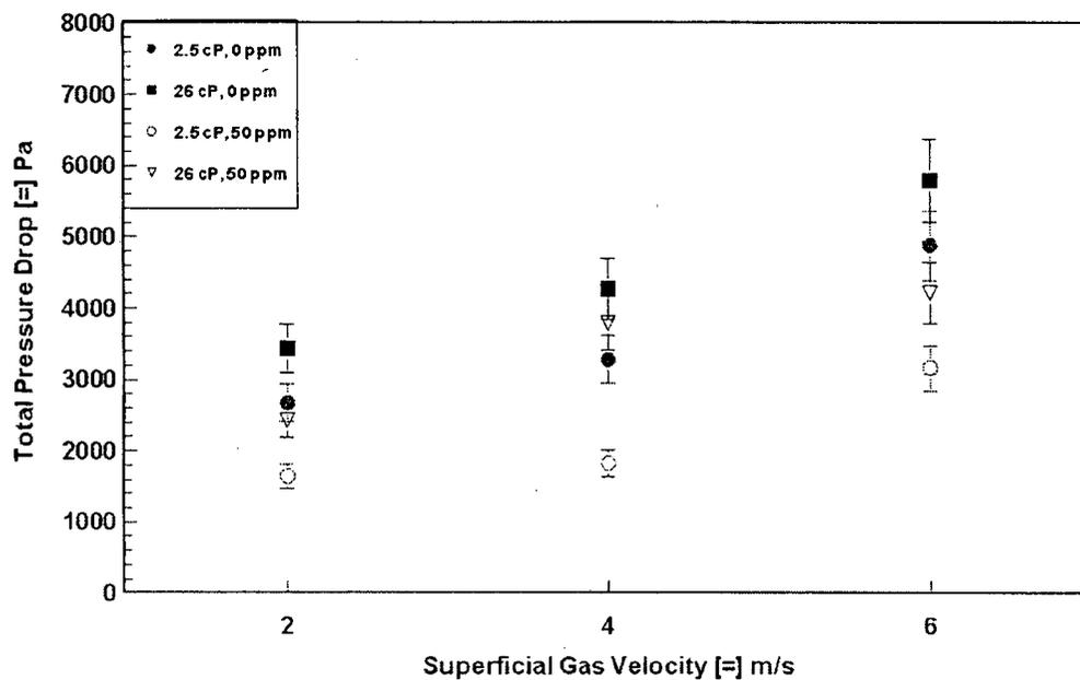
**Figure 9 Effect of Viscosity on Total Pressure Drop**
