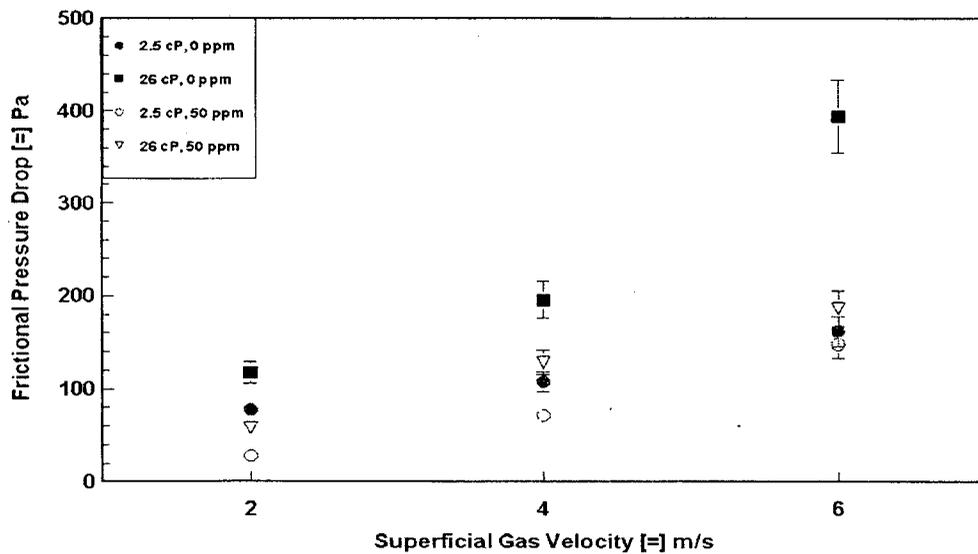
Figure 5 Effect of Viscosity on Frictional Pressure Drop
