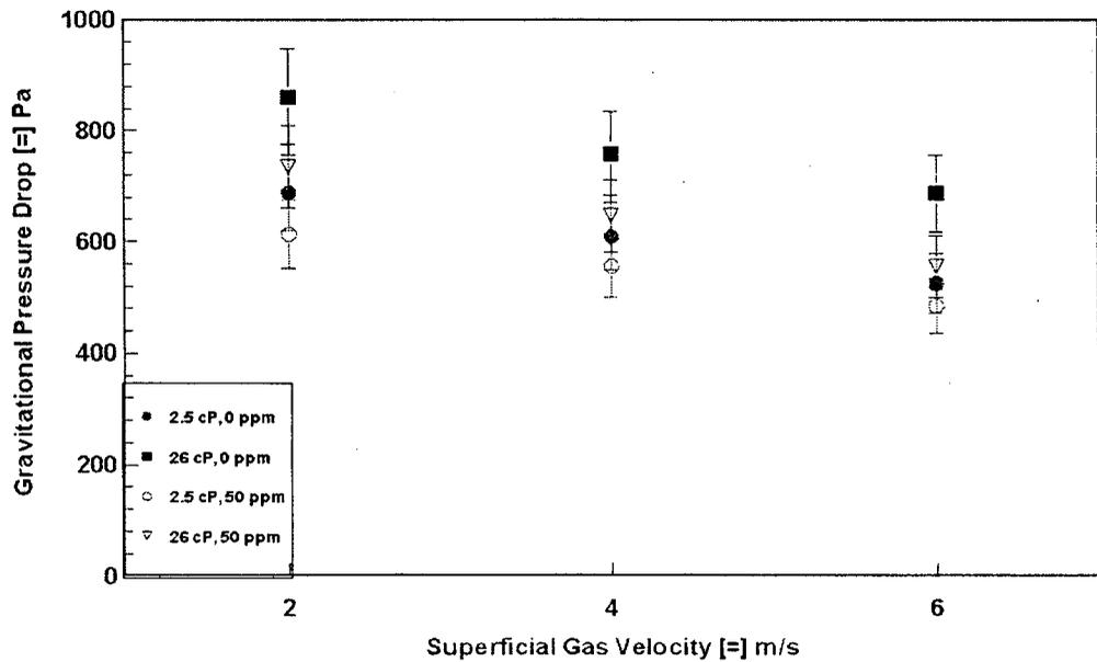
**Figure 7 Effect of Viscosity on Gravitational Pressure Drop
