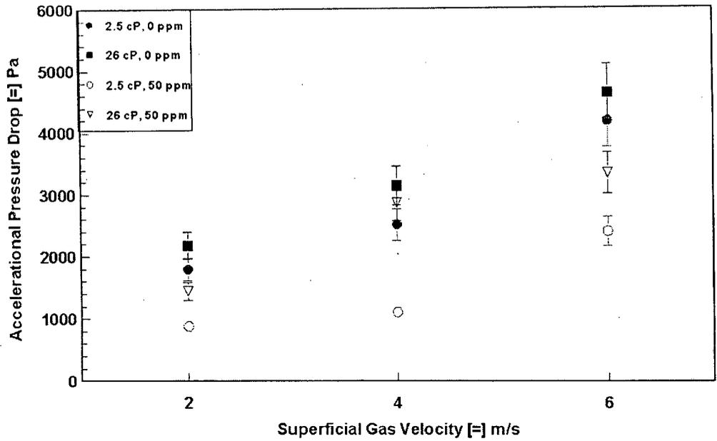
**Figure 6 Effect of Viscosity on Accelerational Pressure Drop
