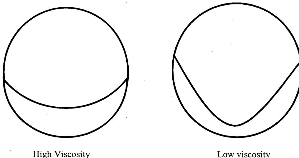
**Figure 3 Surface of liquid film after addition of DRA**
