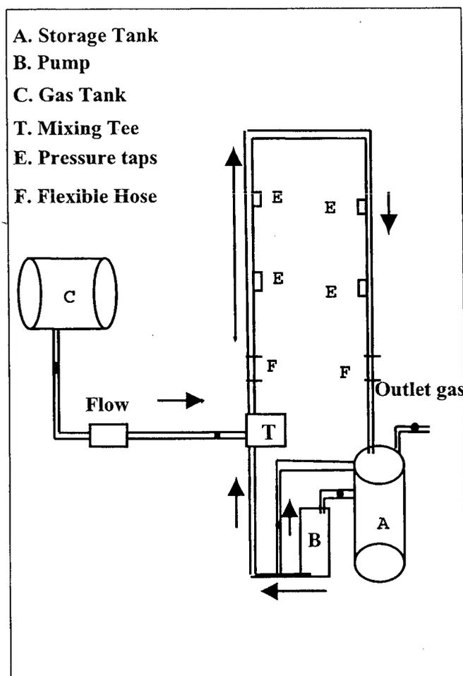
Figure 1 Experimental setup
