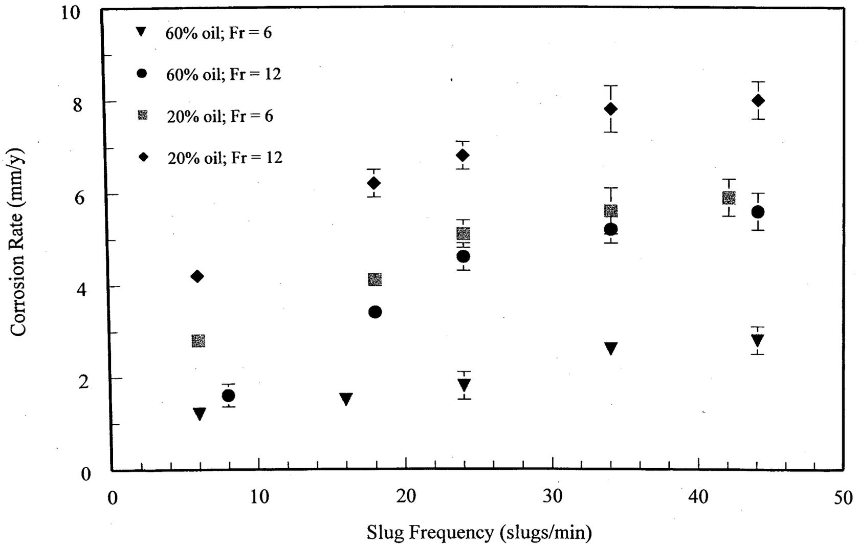
**Figure 10: Corrosion Rate vs. Slug Frequency for 2°; 0.27 MPa**
