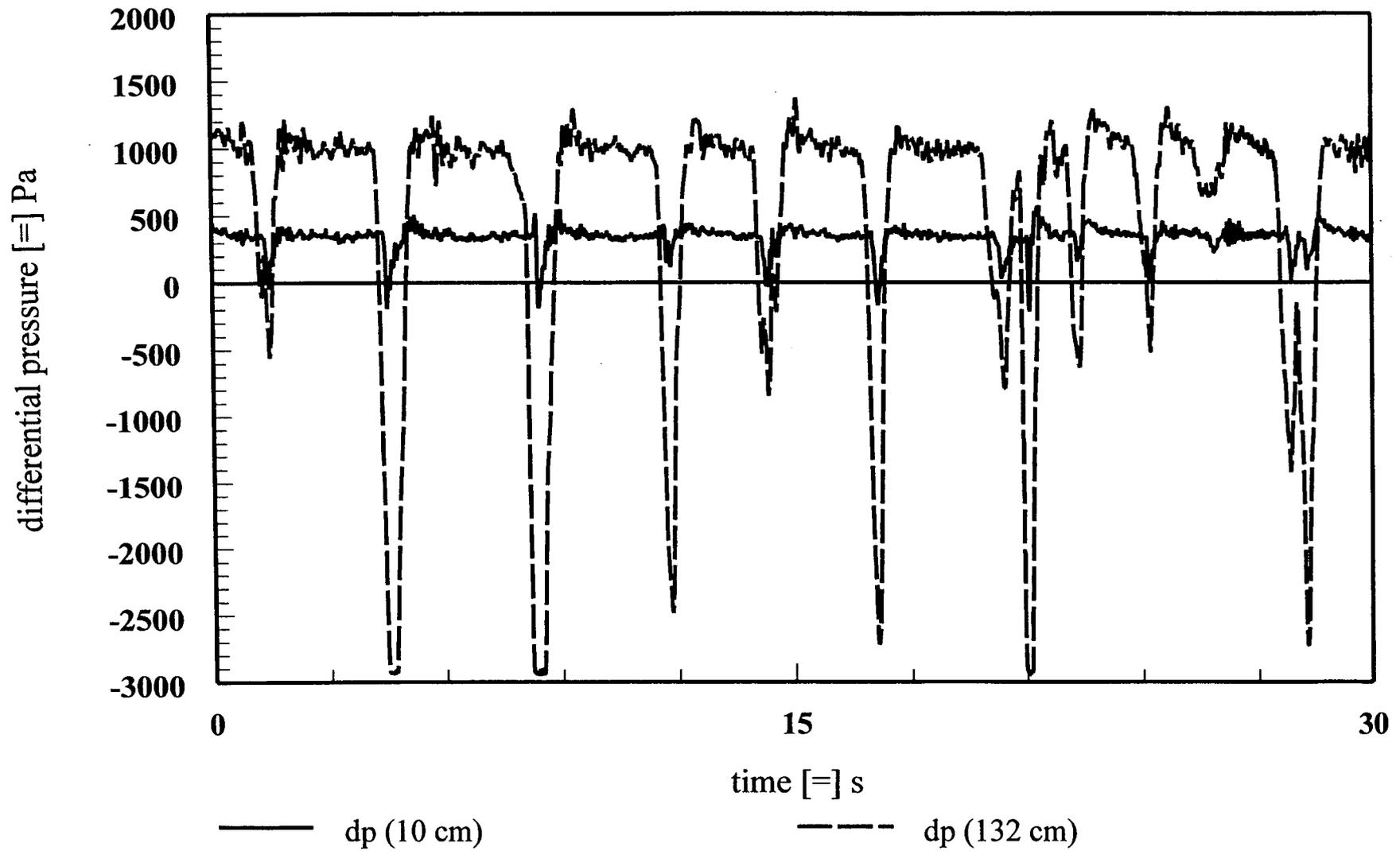
**Figure 3: Sample Differential Pressure Trace for Slug Flow**
