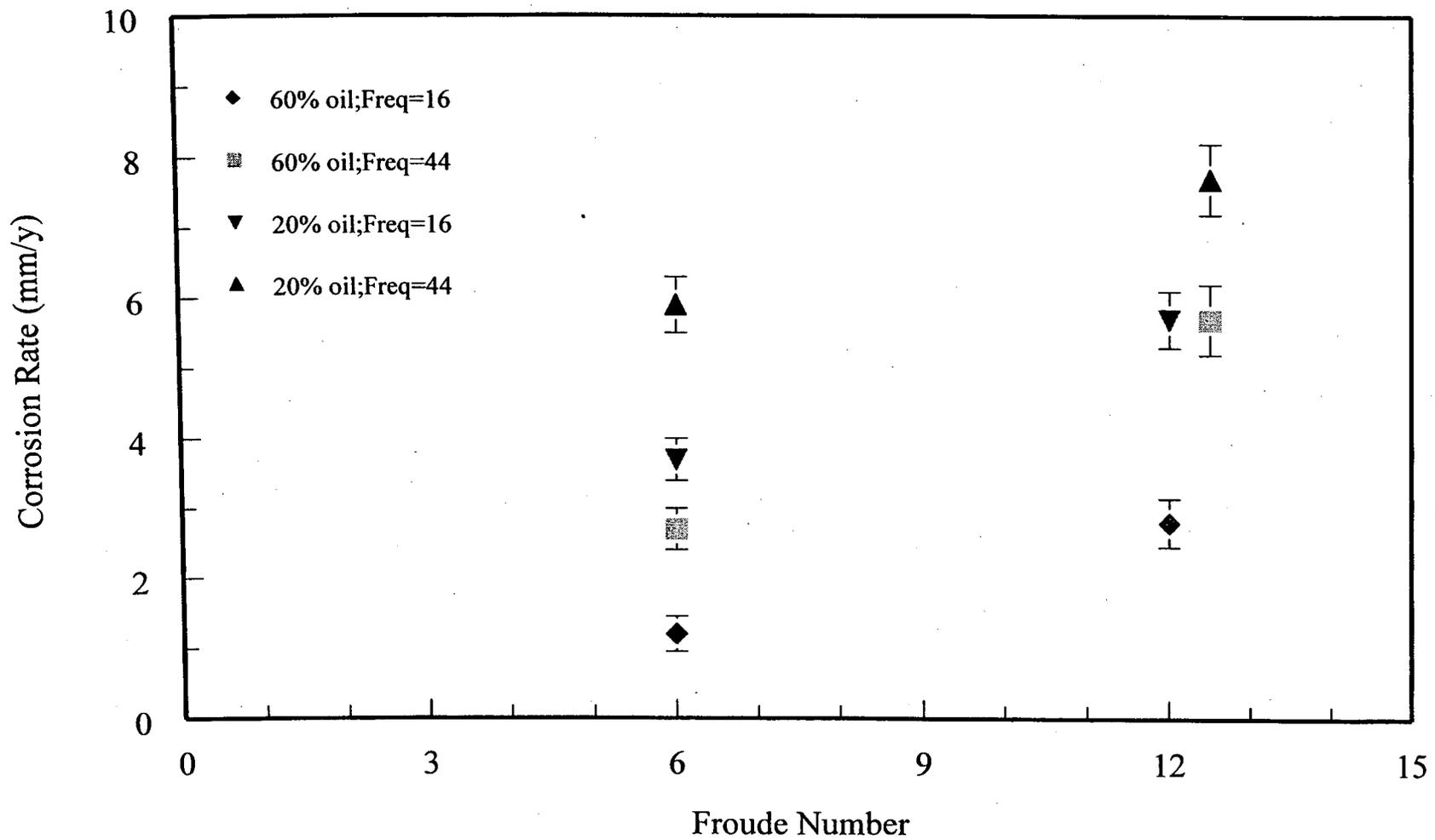
**Figure 11: Corrosion Rate vs. Froude Number for 5°, 0.27 MPa; 80 & 40% saltwater**
