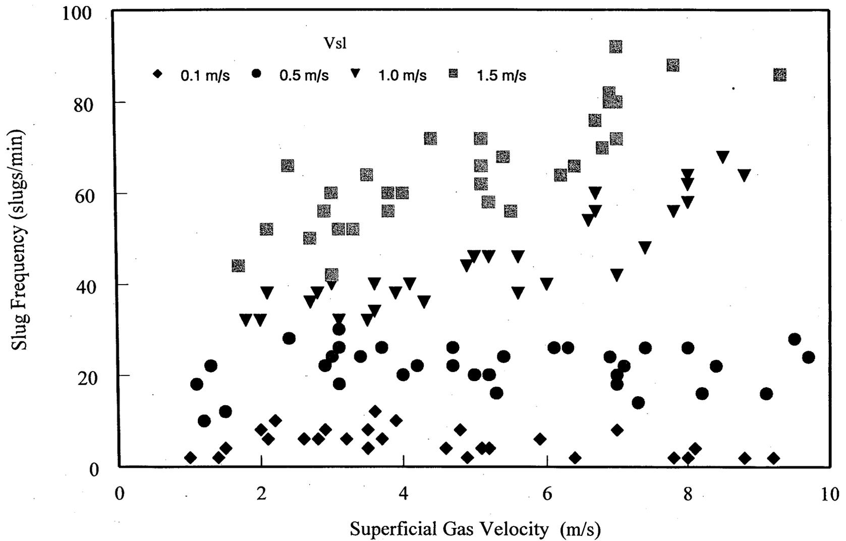
**Figure 5: Slug frequency results @ 5° for all pressure and compositions**
