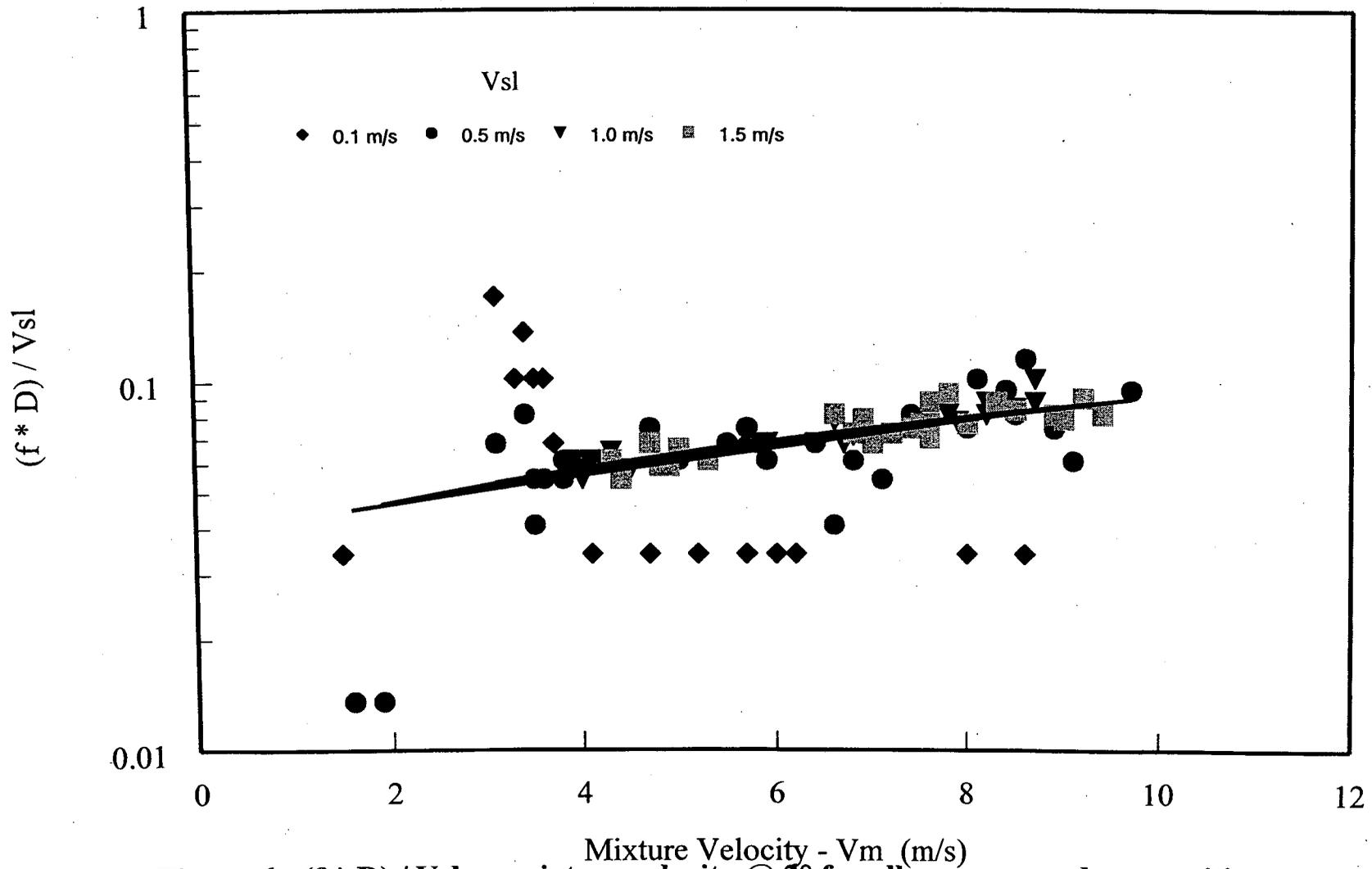
**Figure 6:  $(f * D) / Vsl$  vs. mixture velocity @  $2^\circ$  for all pressure and compositions**
