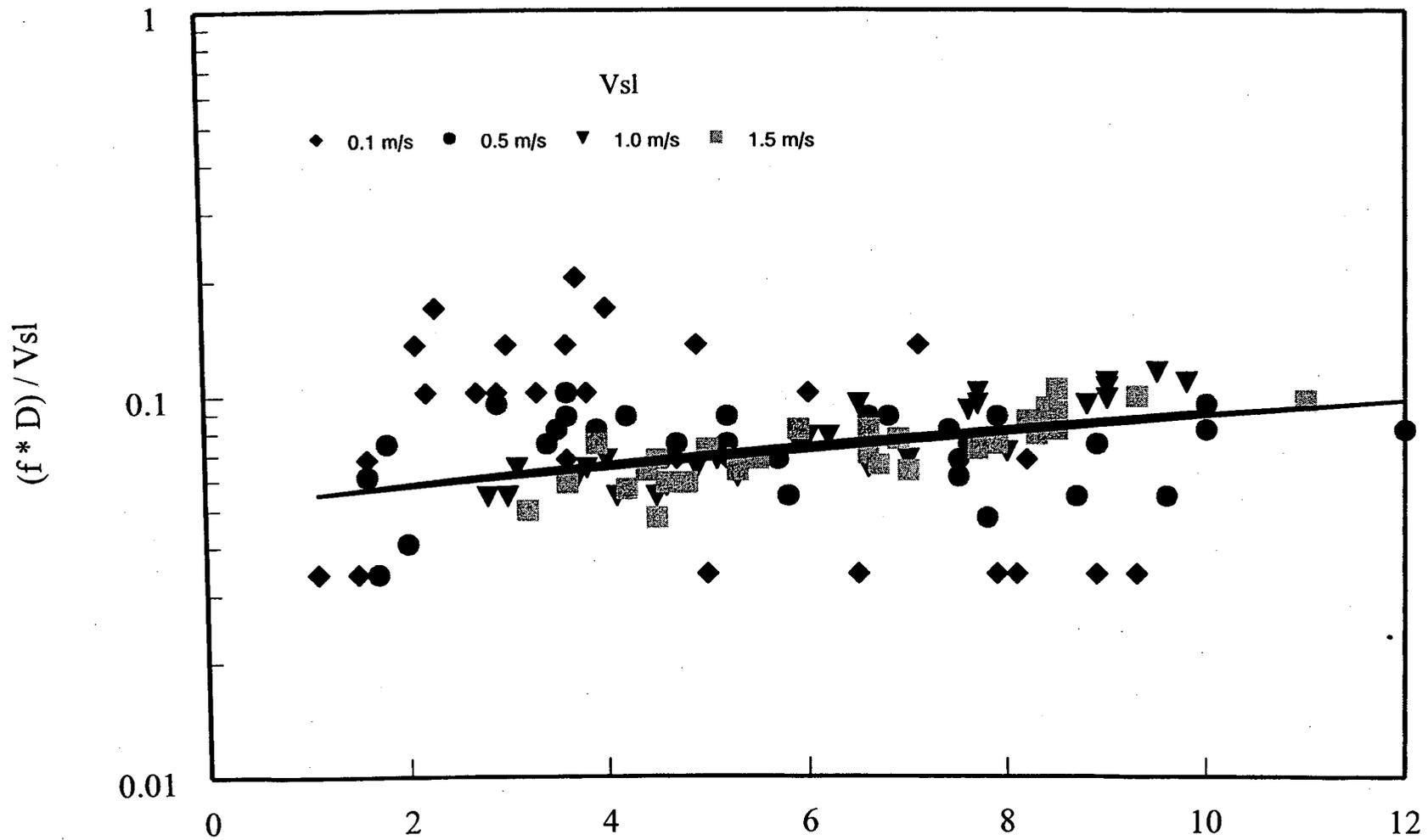
Figure 7:  $(f * D) / V_{sl}$  vs. mixture velocity @ 5° for all pressure and compositions
