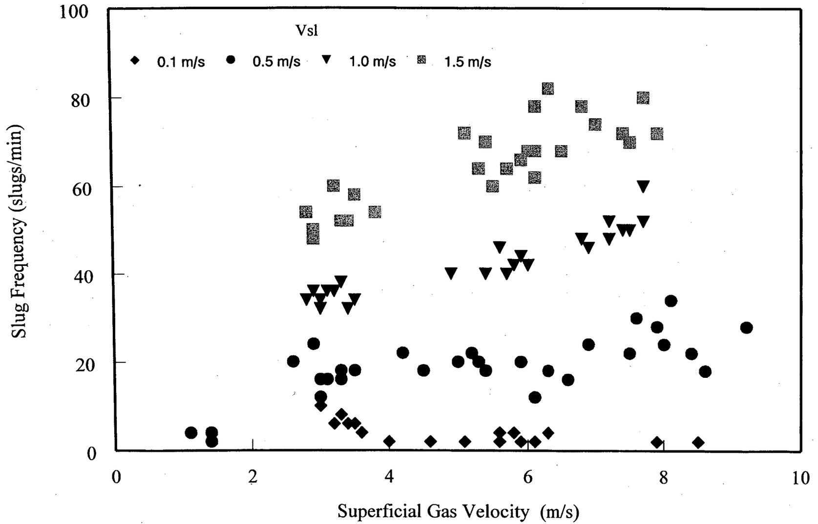
**Figure 4: Slug frequency results @ 2° for all pressure and compositions**
