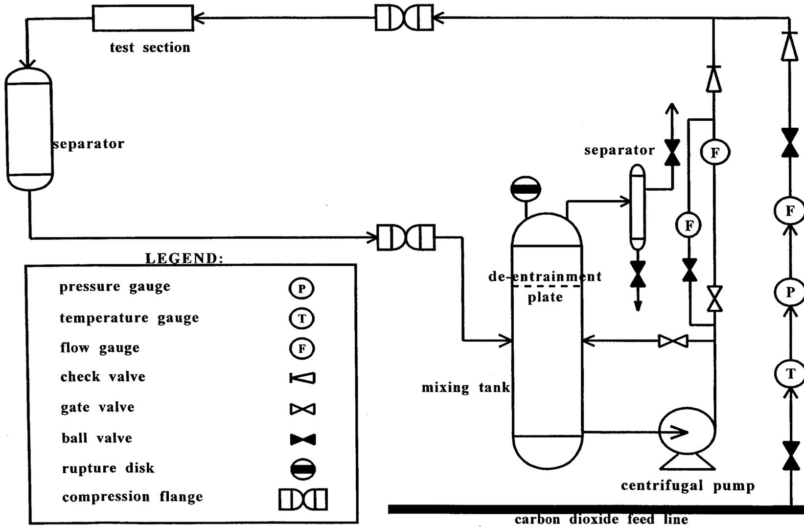
Figure 1: High-pressure, inclinable flow system process flowsheet.
