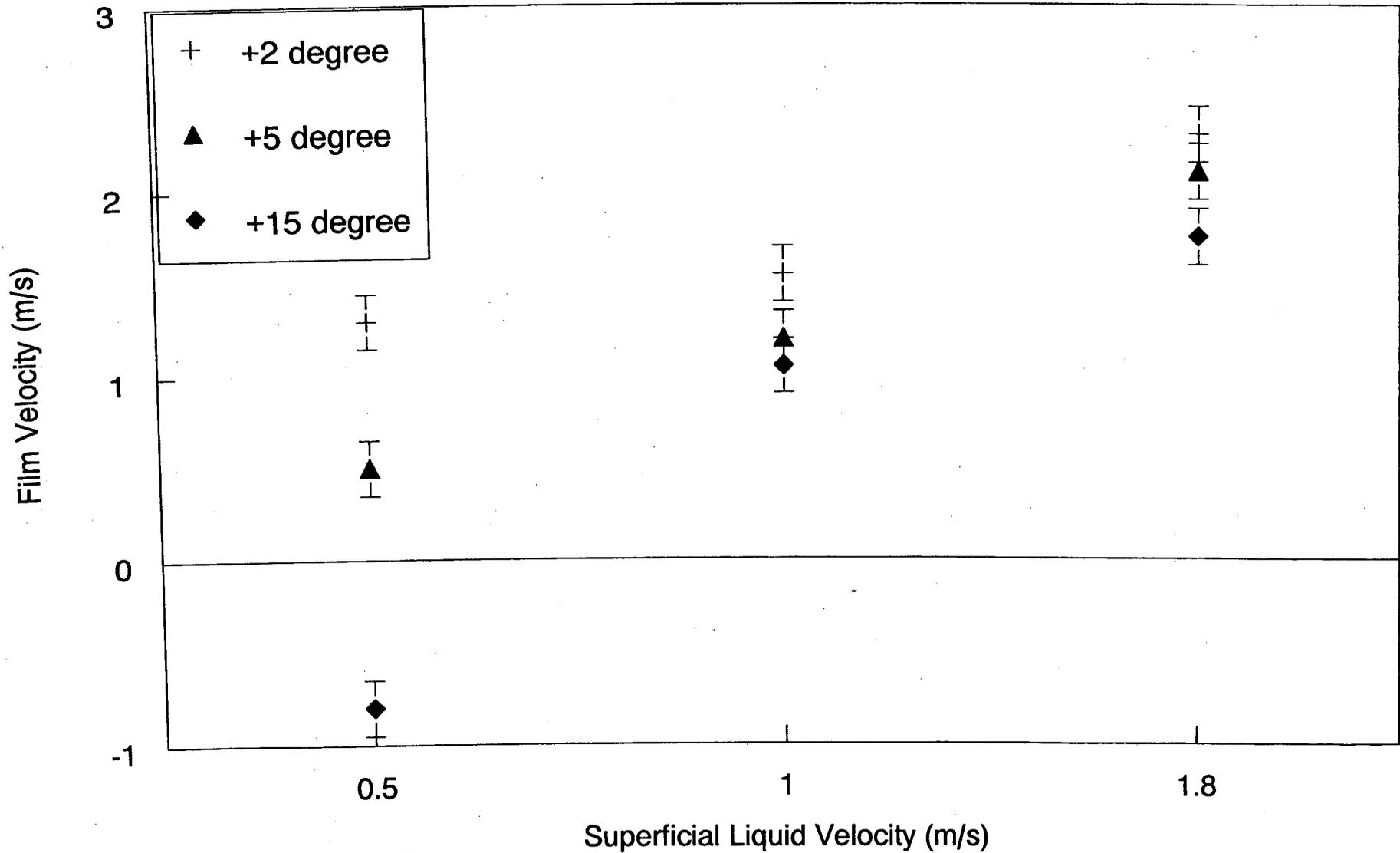
**Figure 9: Effect of Inclination on Film Velocity**
