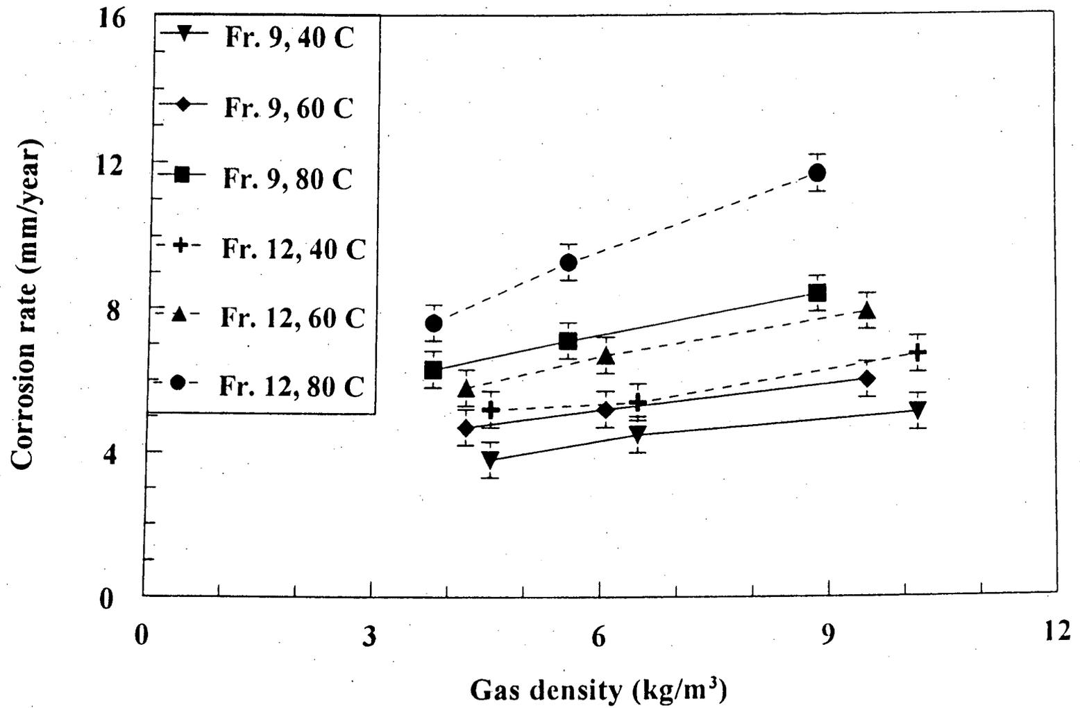
Figure 8: Variation of corrosion rate with gas density at constant CO<sub>2</sub> partial pressure of 0.27 MPa and 40% water cut
