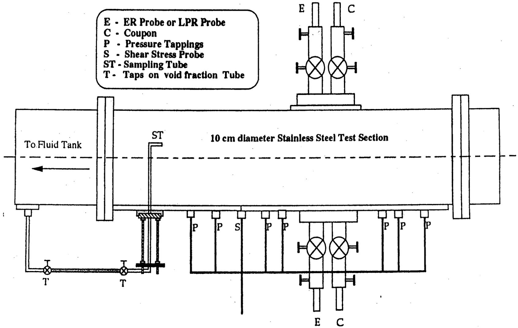
Figure 2: Test Section
