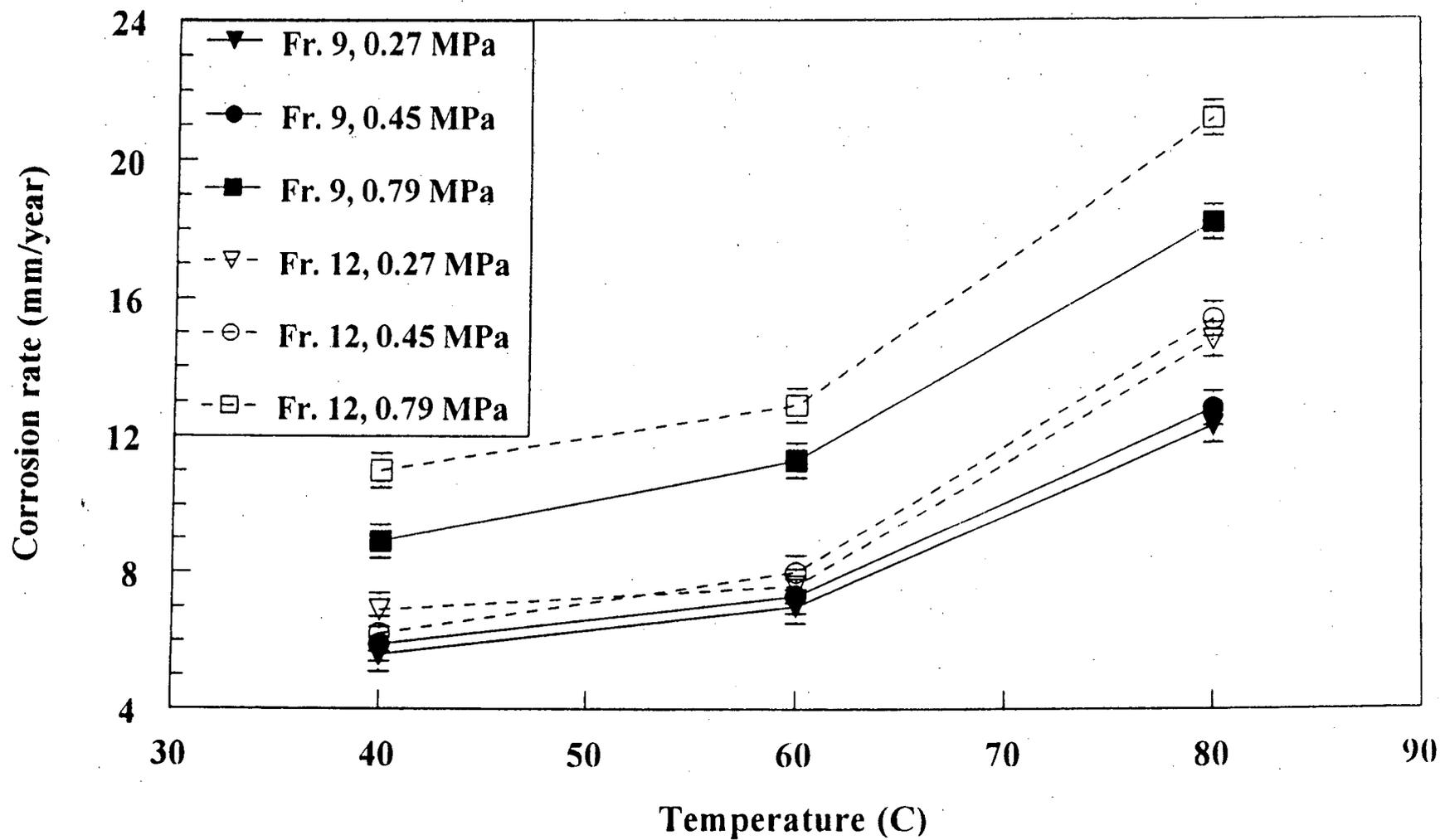
Figure 5: Variation of corrosion rate with temperature at constant CO<sub>2</sub> partial pressure of 0.27 MPa and 80% water cut
