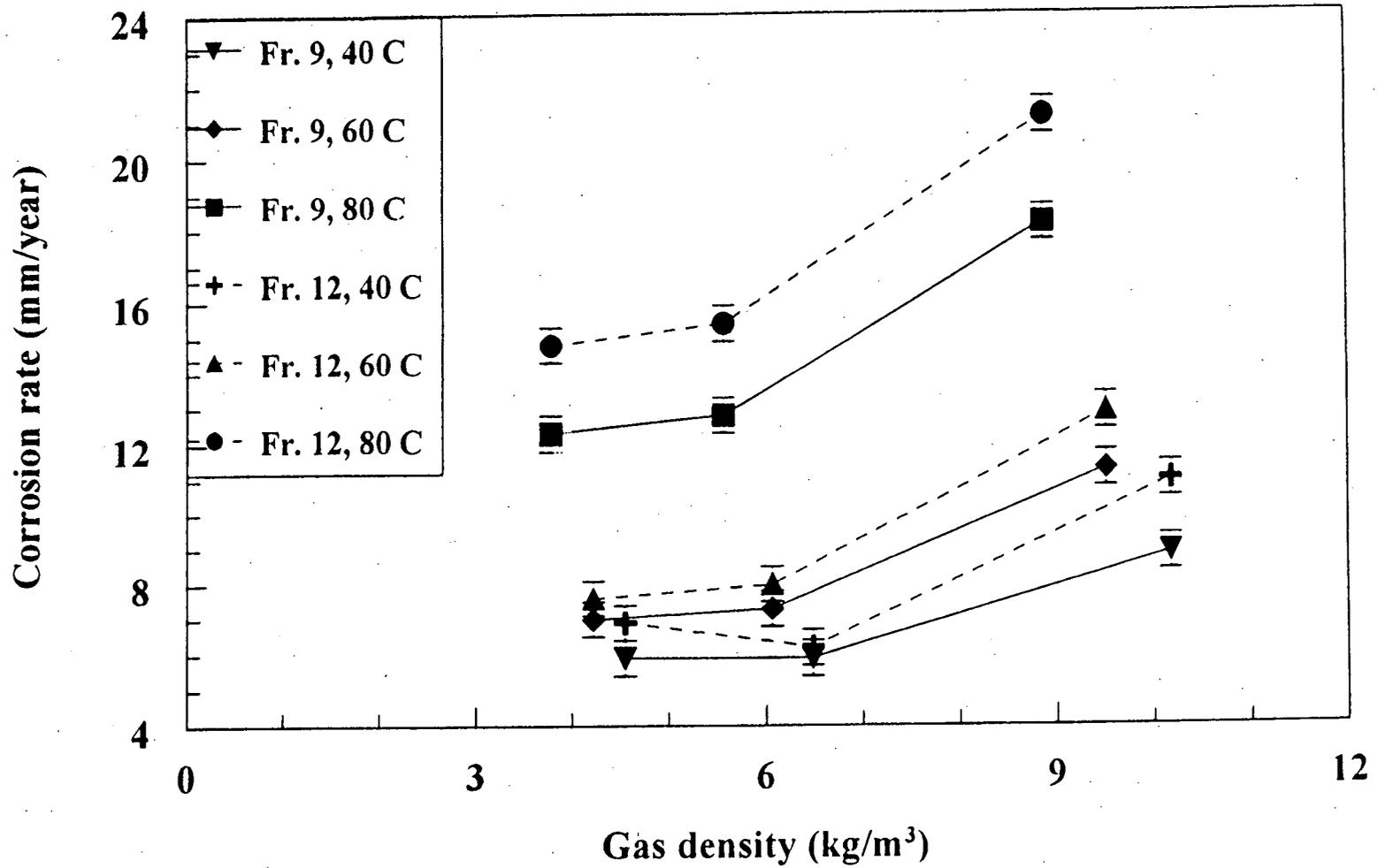
Figure 7: Variation of corrosion rate with gas density at constant CO<sub>2</sub> partial pressure of 0.27 MPa and 80% water cut
