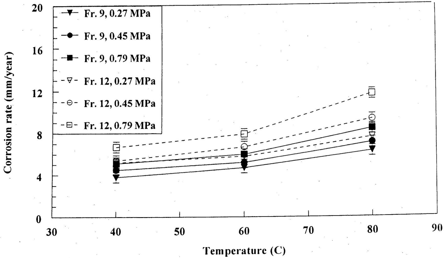
Figure 6: Variation of corrosion rate with temperature at constant CO<sub>2</sub> partial pressure of 0.27 MPa and 40% water cut
