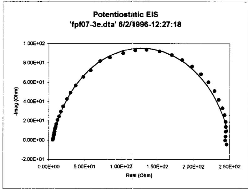
**Figure 9. The impedance spectra of EIS for 0.75 m/s full pipe flow**
