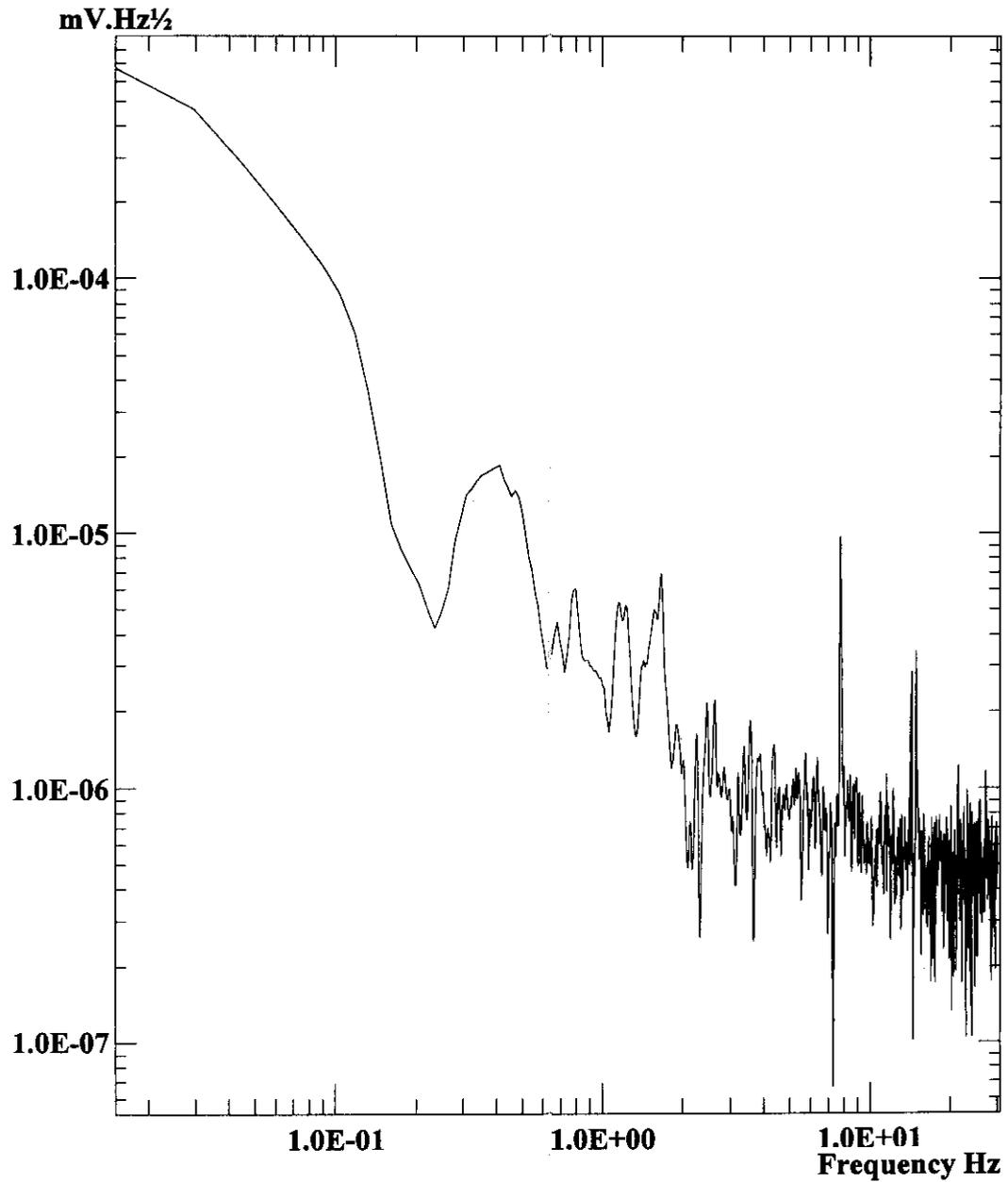
**Figure 7. Potential amplitude spectrum for Froude No. 6 stationary slug flow
