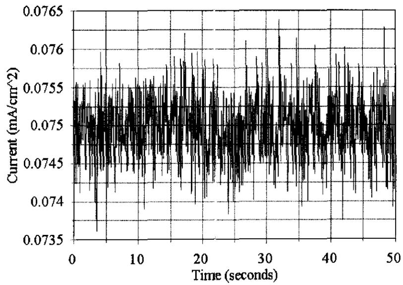
Figure 4. Voltage & current noise response for 1.1 m/s full pipe flow .
