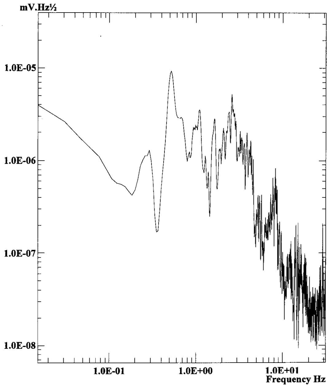
**Figure 15. Potential amplitude spectra for Froude number 6 stationary slug flow
