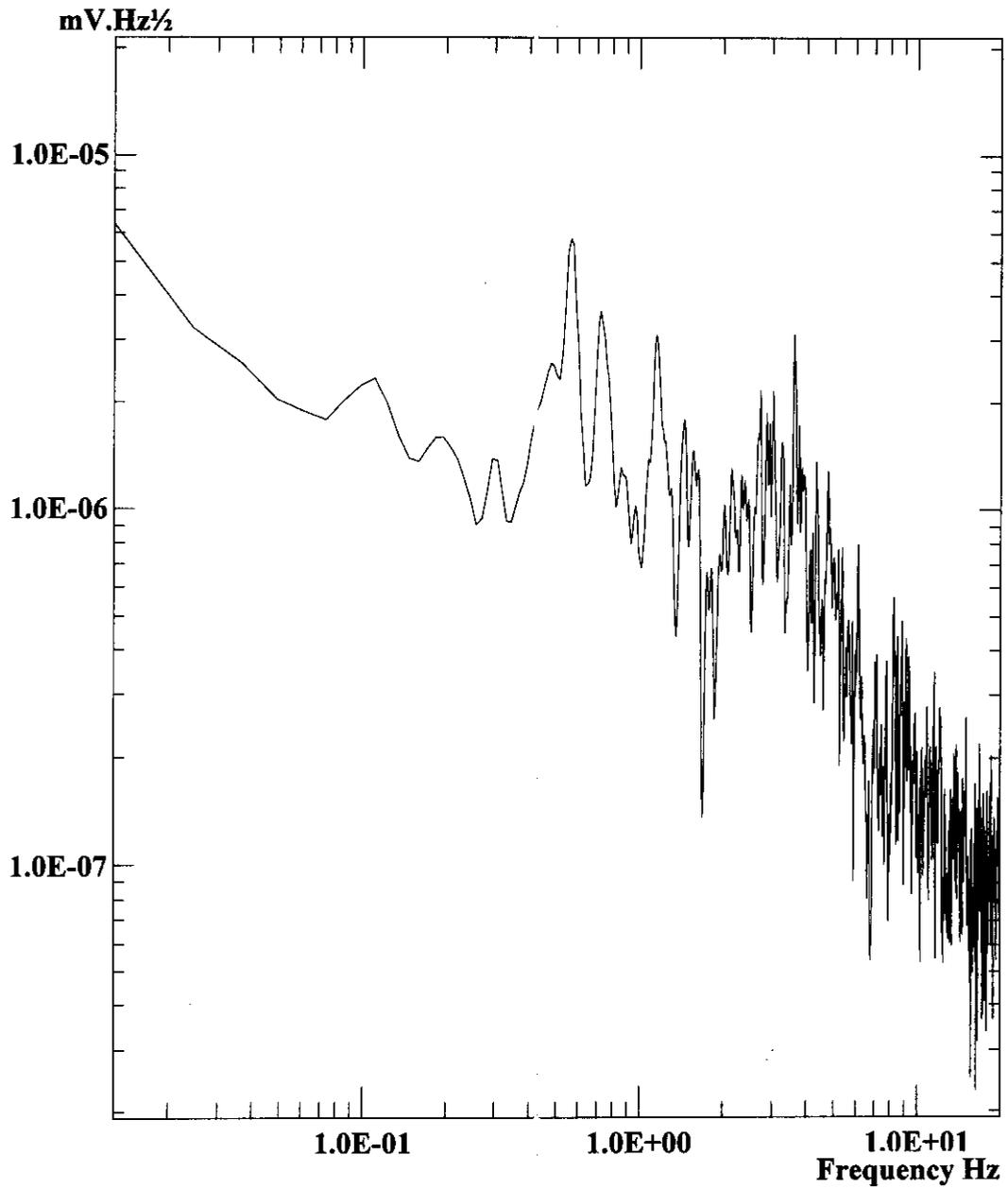
**Figure 8. Potential amplitude spectrum for Froude No. 6 stationary slug flow
