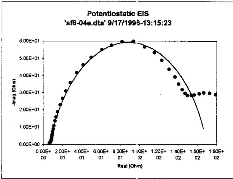
**Figure 10. The impedance spectra of EIS for Froude No. 6 stationary slug flow**
