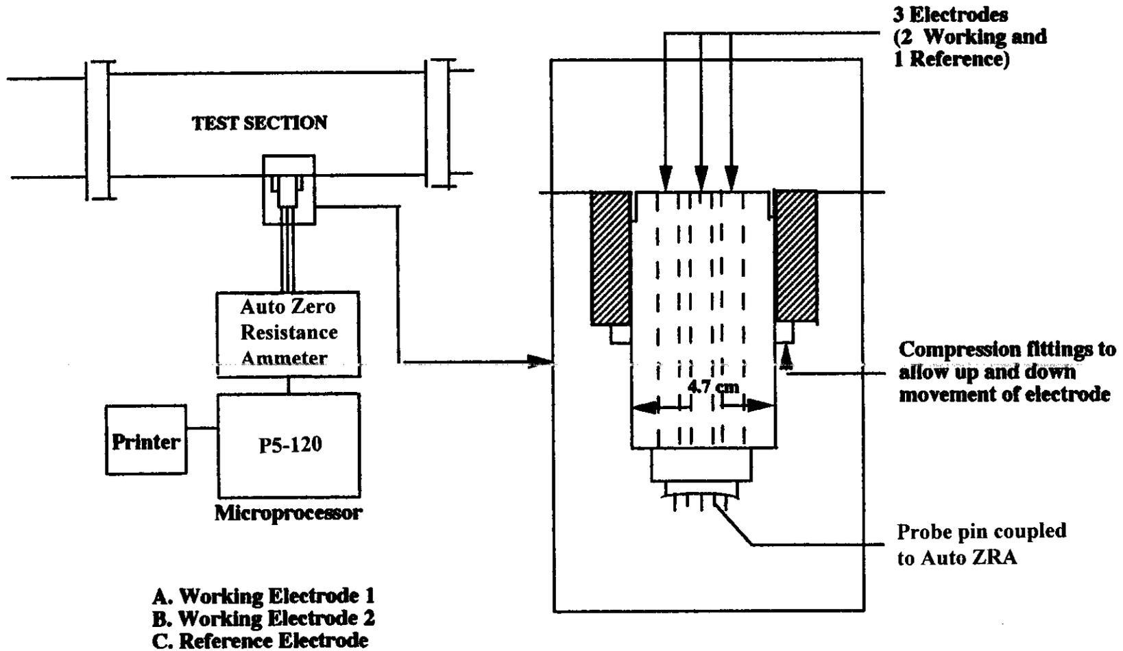
Figure 3.1 Data logging section
