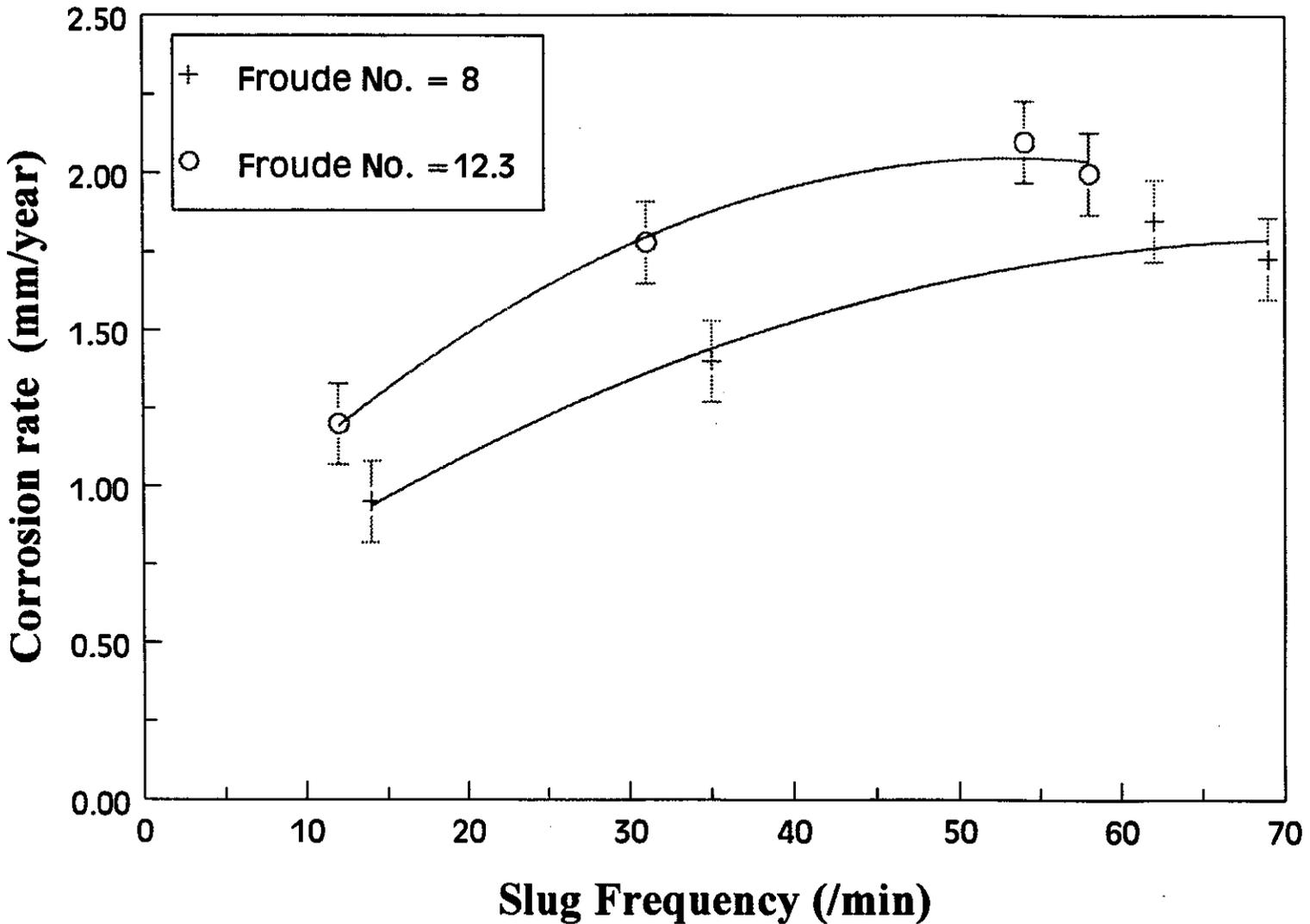
**Figure 3 Corrosion rate vs Slug Frequency**
