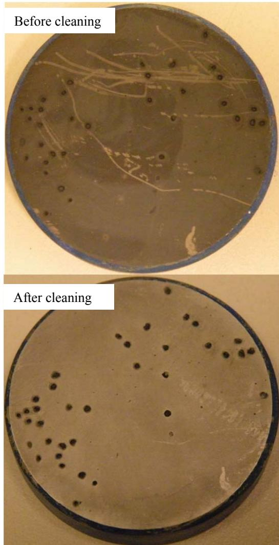
Figure 6.24 Views of the experiment sample #2 after 34 days exposure with corrosion product layers (left) and without corrosion product layers (right) at test conditions 25°C, pH 5, 1 wt% NaCl solution saturated with CO<sub>2</sub>.
