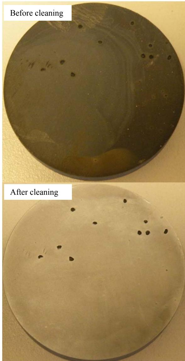
Figure 6.19 View of the experiment sample #1 after 25 days exposure with corrosion product layers and without corrosion product layers at test conditions 25°C, pH 5, 1 wt% NaCl solution saturated with CO<sub>2</sub>.
