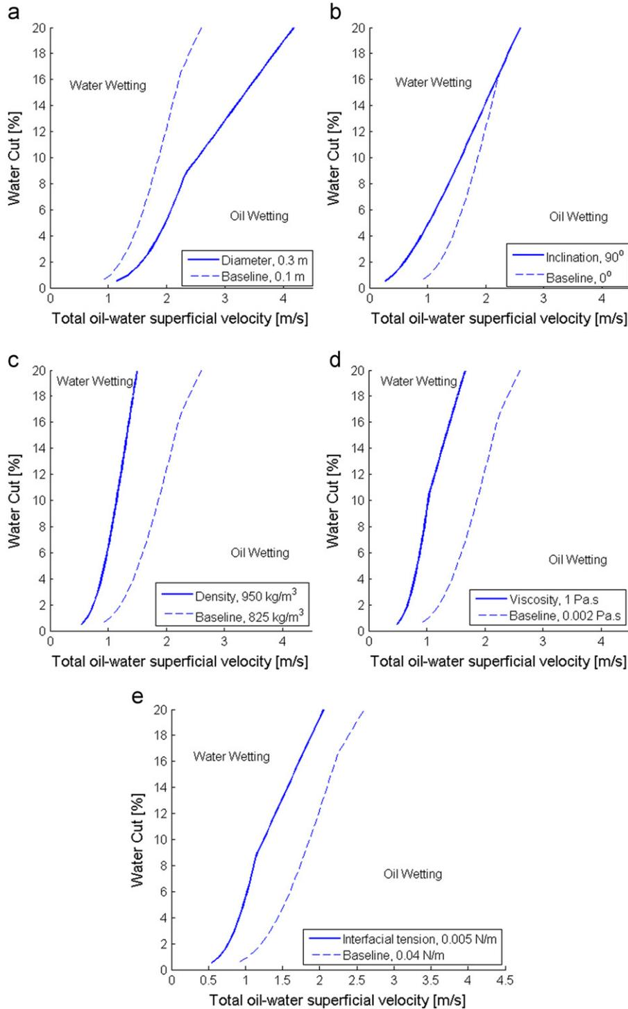
**Fig. 2.** Predicted transitions between oil and water wetting. All of the graphs have one common set of conditions: “Baseline” (0.1 m horizontal pipe, density 825 kg/m<sup>3</sup>, viscosity 0.002 Pa s, interfacial tension 0.04 N/m). The deviation from the baseline is for (a) larger pipe diameter (0.3 m), (b) vertical inclination (90°), (c) higher density (950 kg/m<sup>3</sup>), (d) higher viscosity (1 Pa s) and (e) lower interfacial tension (0.005 N/m).
