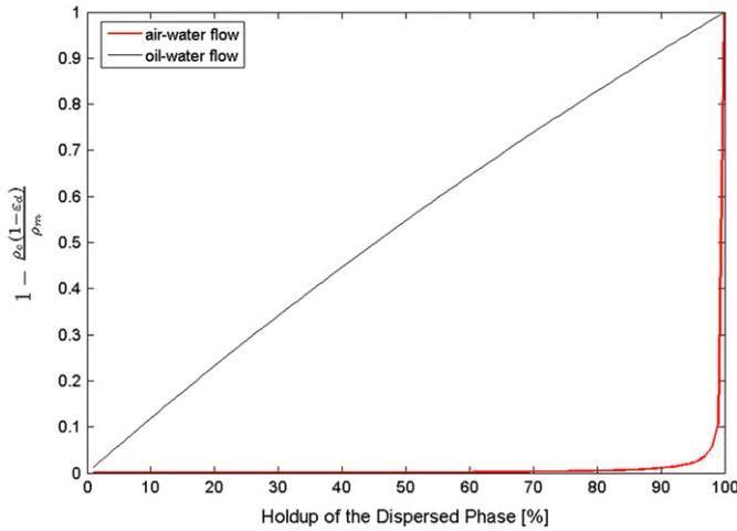
**Fig. 1.** Criterion for dilute dispersions for air–water and oil–water two phase flows. The criterion is valid when  $1 - \rho_c(1 - \varepsilon_d)/\rho_m \cong 0$ , and is drawn up for  $\rho_{air} = 1.2 \text{ kg/m}^3$ ,  $\rho_{water} = 1000 \text{ kg/m}^3$  and  $\rho_{oil} = 825 \text{ kg/m}^3$ .
