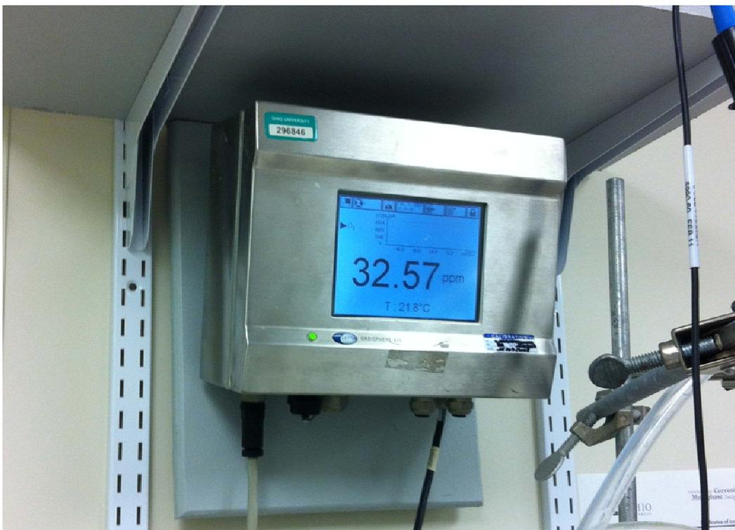
Figure 11. Oxygen meter, Orbisphere 410.
