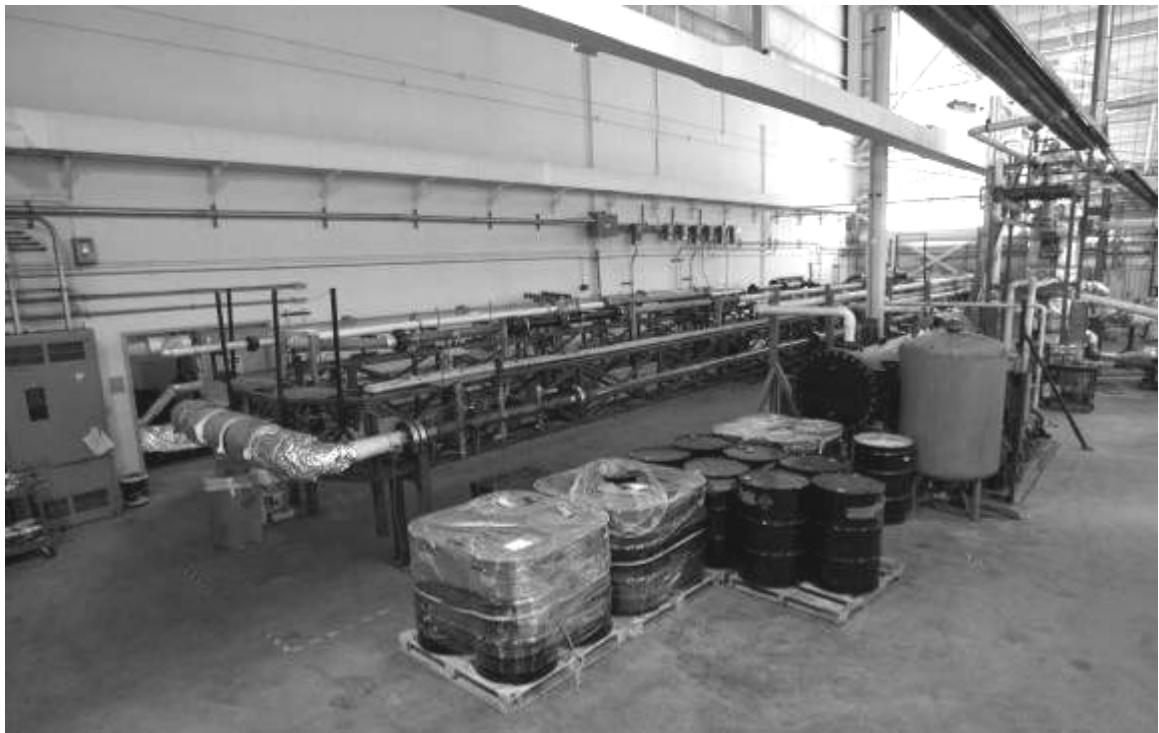
Figure 68. Picture of the flow loop in horizontal position.
