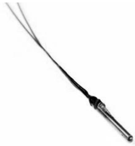
*Figure 66.* One conductivity probe, 160 conductivity probes are used in the doughnut cell.
