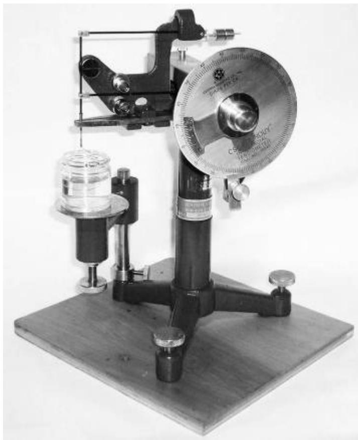
*Figure 57.* Platinum ring tensiometer used in these experiments.
