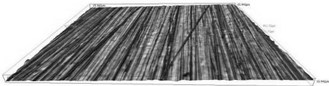
Figure 60. 3D picture of the metal surface after polishing with 600 grit sandpaper, roughness:  $1.1 \mu\text{m}$ .
