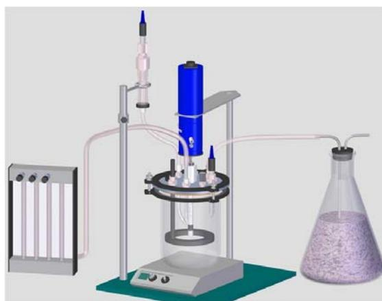
**FIGURE 1 – Experimental Setup for Corrosion Tests**
