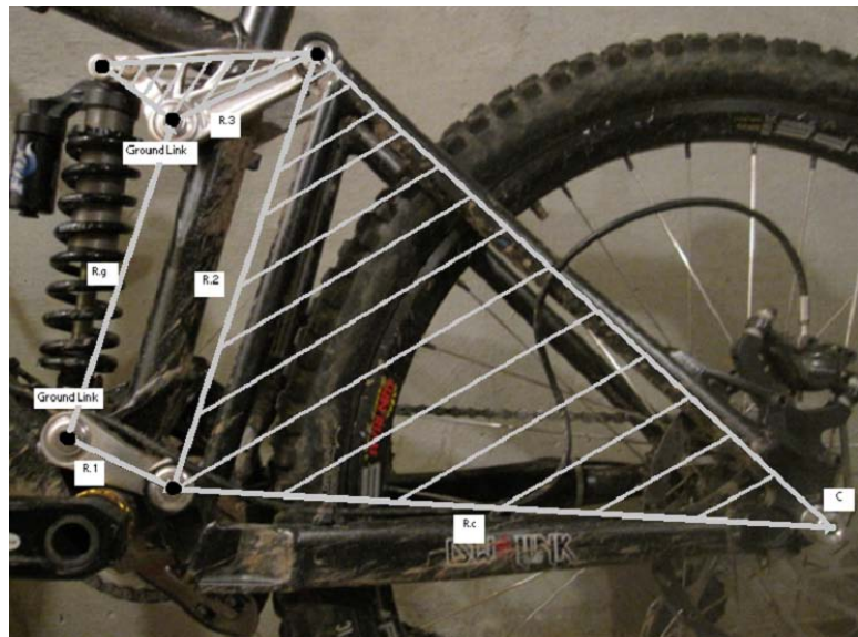
Mountain Bike Rear Suspension Mechanism
