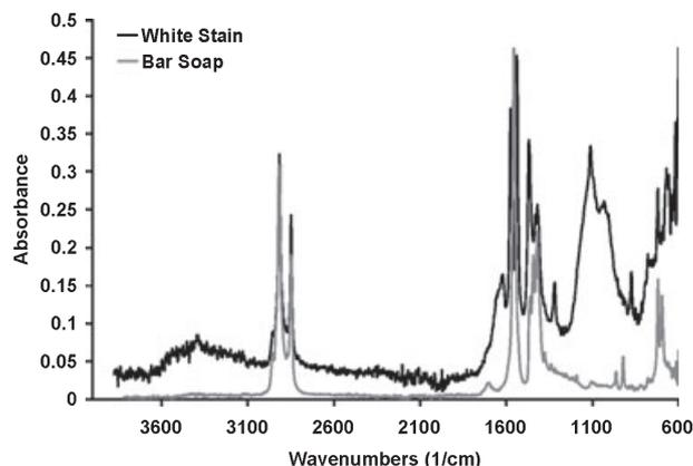
FIG. 4—FTIR spectra of (■) the light sample and (■) commercial bar soap.
