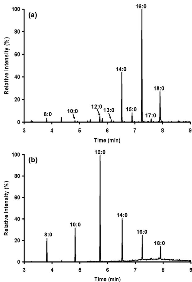
FIG. 6—Selected ion monitoring (SIM) chromatograms of  $m/z$  87 for (a) the light sample and (b) commercial bar soap.
