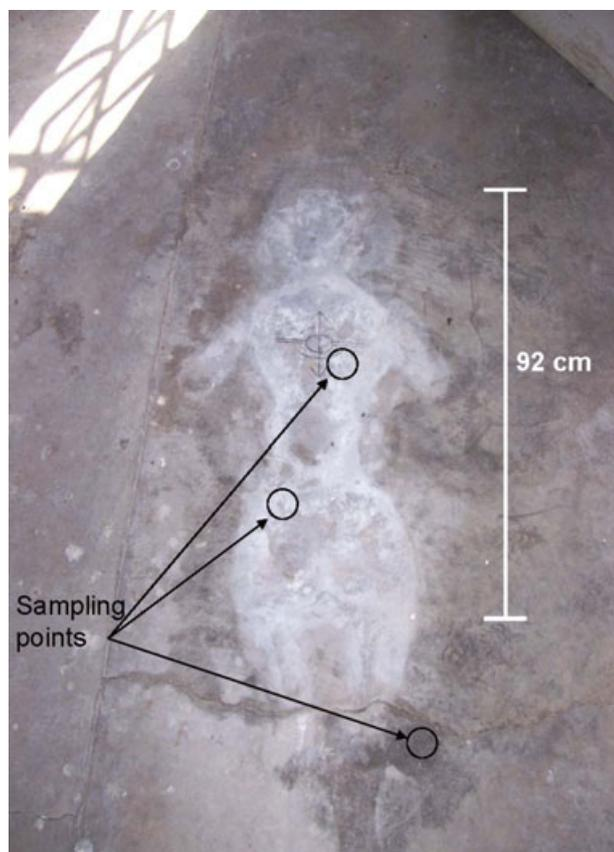
FIG. 1—Photograph of the questioned stain on the concrete floor showing the light area surrounded by a darker border.
