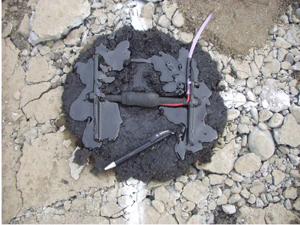
FIGURE 8 Placement of Strain Gage on Mastic.
