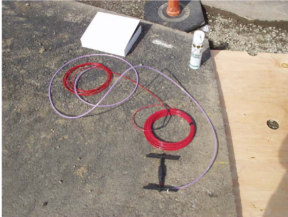
FIGURE 6 Strain Gage with Protective Nylon Sheath.
