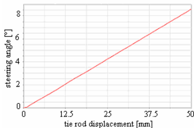
FIGURE 13 Tire steering angle as a function of tie rod displacement.
