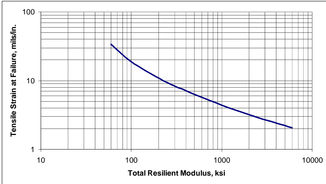
Figure 6 Relationship between modulus and tensile strain at failure to estimate the fatigue strength of HMA mixtures (Von Quintus, et al., 2001).
