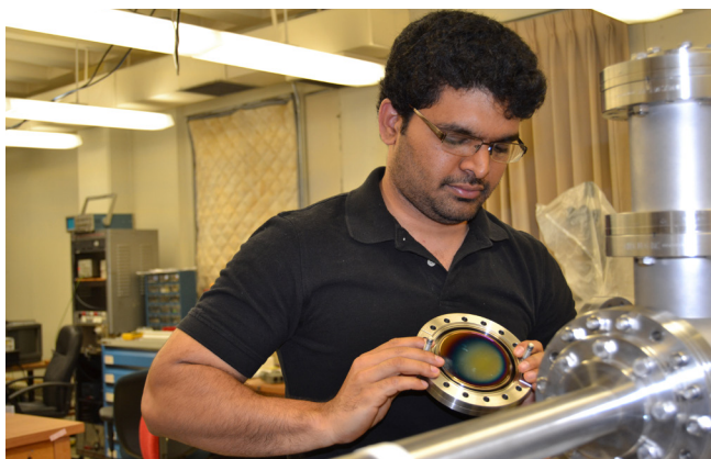
Pratheesh Jakkala, a doctoral student in physics and astronomy, deposits Indium Gallium Nitride into a radio frequency magnetron sputtering machine used in his solar cell research.
